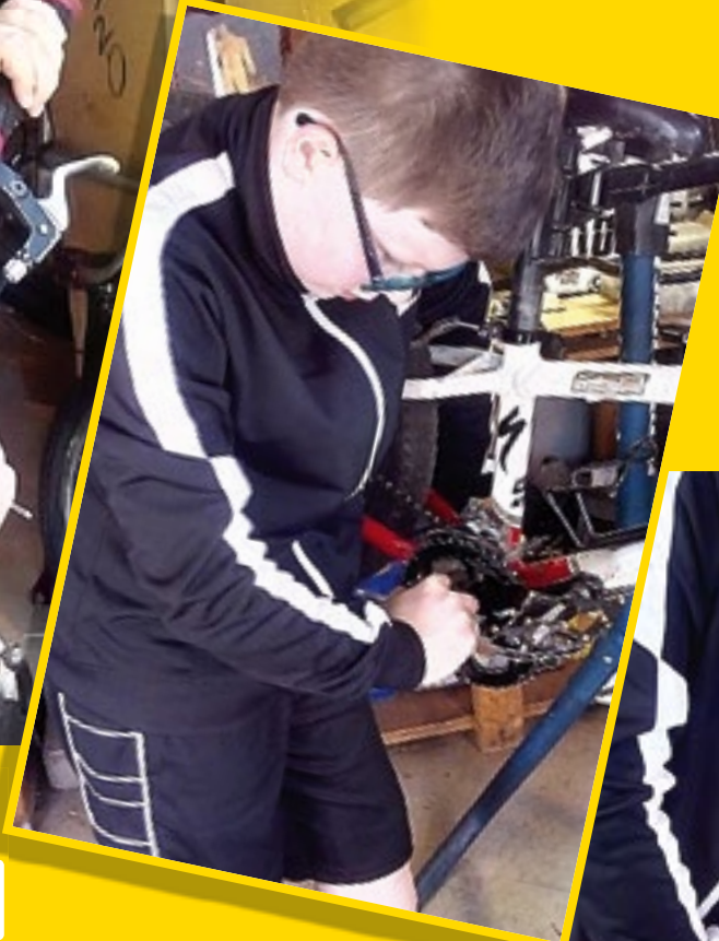
THE AUTHOR'S SON, EWAN, CHECKS HIS HANDLEBAR BOLTS, CHAIN RING BOLTS, AND CRANK ARM BOLTS. JIM MACNAUGHTON
